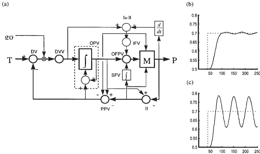
**Figure 11.** Comparison with PID control. (a) The model of Figure 1 represented with control theory notation. Again, the thick lines highlight the kinematic feedback control aspects of the system. (b) Position trace during a reaching movement made with the PPV–OPV pathway intact. (c) Reaching movement made without the PPV–OPV pathway ( $\eta = 0$ ).
