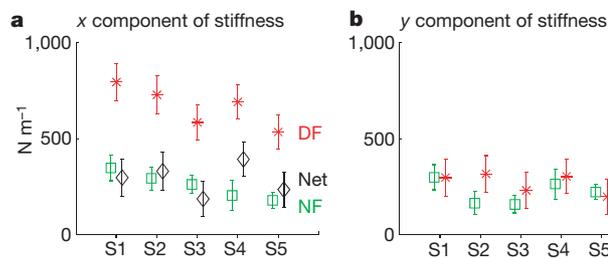
**Figure 4** Stiffness and stability. **a**, The  $x$  components of hand stiffness in the NF (green), hand stiffness in the DF (red) and net stiffness of the hand and DF environment (Net, black) after learning. Vertical bars show 90% confidence intervals. **b**, The  $y$  components of hand stiffness in the NF (green) and in the DF (red).
