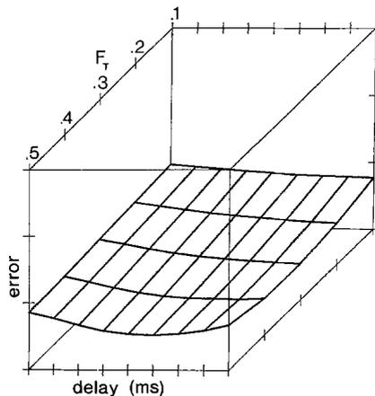
**Fig. 9.** Dependence of time-weighted velocity error on the feedback delay ( $\tau$ ) for position (left panel) and torque feedback (right panel). Feedback delay varied from 4 to 100 ms in 12 ms increments and the values of the feedback coefficients are indicated in the figure. The figure depicts average values of the normalized error for ten different experimental conditions (five values of elbow flexion ranging from 30° to 150° and forces applied to the forearm or the upper arm)
