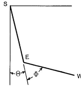
Fig. 1. Schematic of the human arm. S, E, and W denote shoulder, elbow and wrist connected by rigid links.  $\theta$  corresponds to the angle of forward flexion at the shoulder and  $\phi$  the angle of elbow flexion
