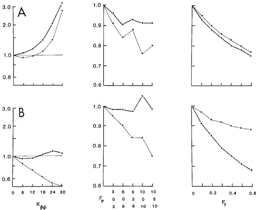
**Fig. 11 A, B.** Effect of different parameter values of cross-coupling stiffness ( $K_{\theta\phi}$ ), position feedback ( $F_p$ ) and torque feedback ( $F_T$ ) on normalized error resulting from a force perturbation applied to the upper arm (A) or to the forearm (B) during a pointing movement. The normalized error was computed in two ways: deviation of wrist from its reference trajectory (*light traces*) and sum of the deviations of angular velocities (*heavy traces*)
