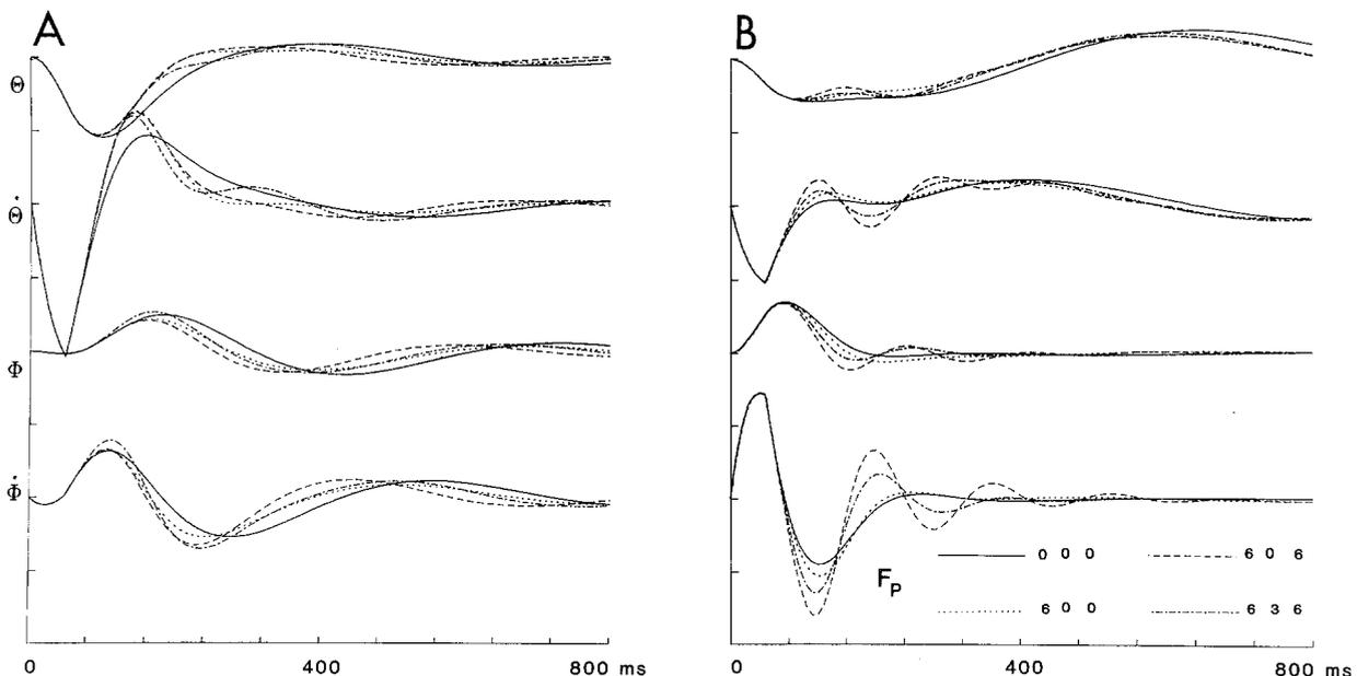
**Fig. 4A, B.** Effect of different combinations of position feedback on the response to a force perturbation to the upper arm. In A, the forearm was flexed ( $\phi = 135^\circ$ ) and extended ( $30^\circ$ ) in B. The values of the feedback coefficients  $\{F_{\theta}, F_{\theta\phi}, F_{\phi}\}$  are indicated in the figure
