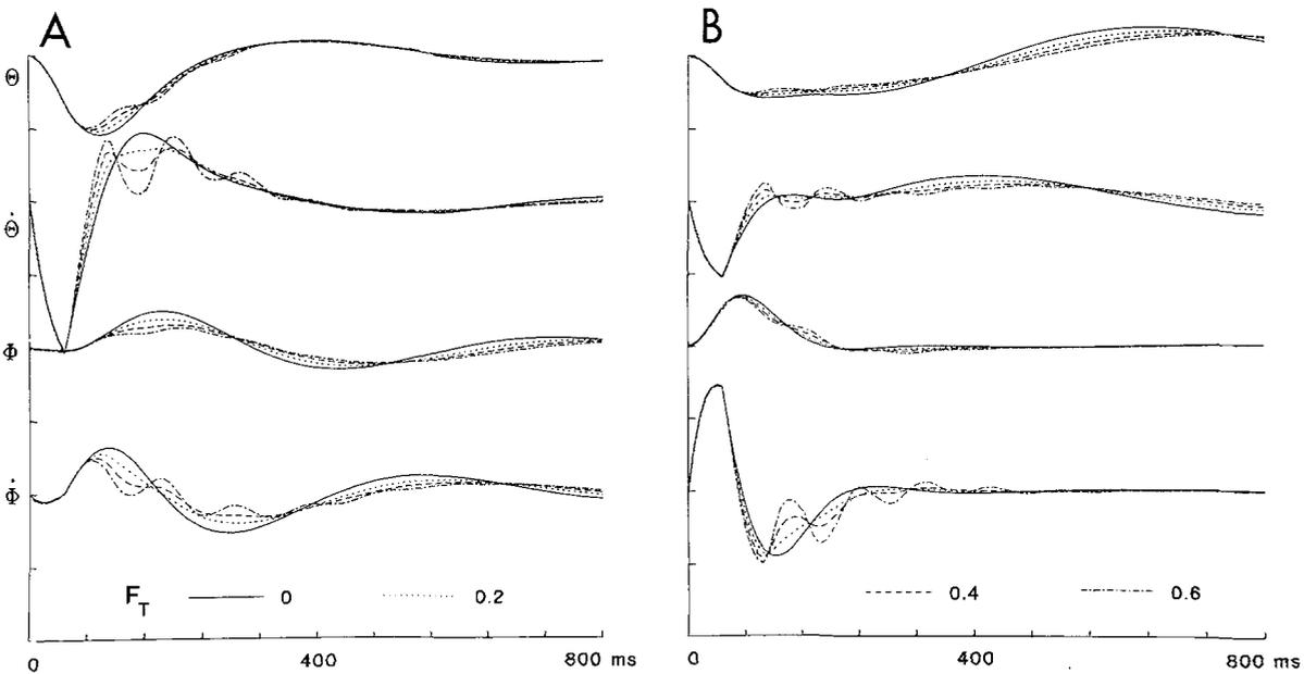
**Fig. 6A, B.** Effect of different values of torque feedback on response to pulse perturbations to the upper arm, with the forearm flexed ( $\phi = 135^\circ$ ) in **A** and extended ( $30^\circ$ ) in **B**
