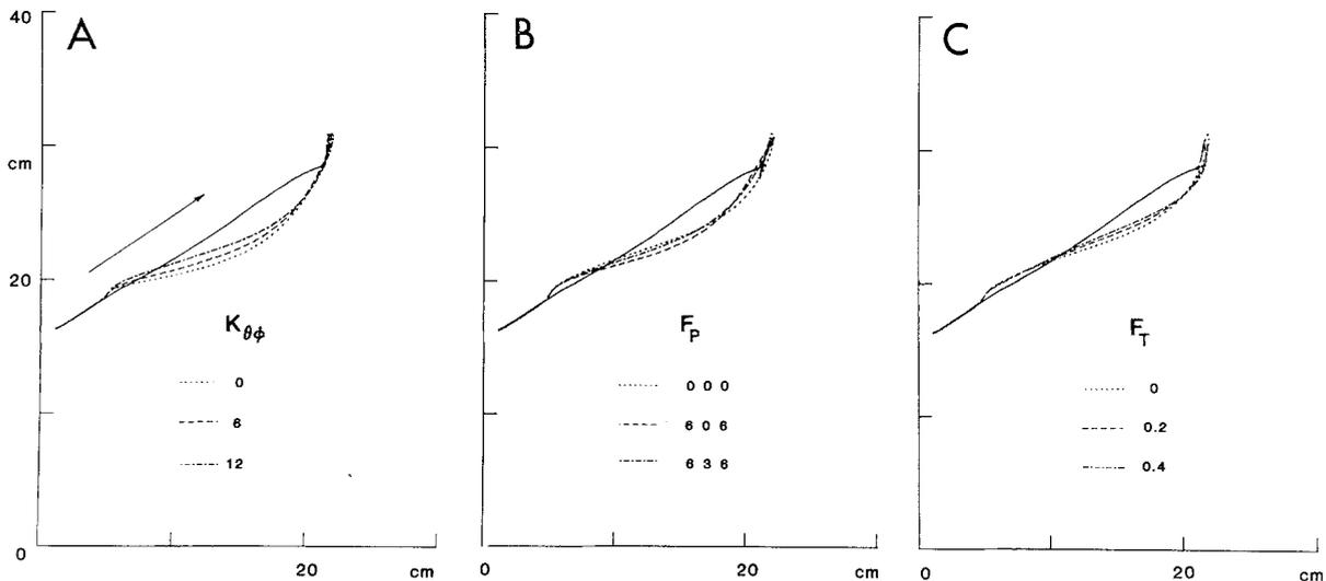
Fig. 10A–C. Effect of perturbations to the upper arm during a pointing movement. Effects of different values of cross-coupling stiffness (A), position feedback (B) and torque feedback (C) are illustrated
