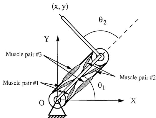
**Fig. 2.** The two-joint arm model. Three pairs of antagonist muscles are included: pair #1 is shoulder muscles, pair #2 is elbow muscles, pair #3 is biarticular muscles. The moment arms of these muscles are assumed to be constant. The elbow and shoulder are assumed to be hinge joints
