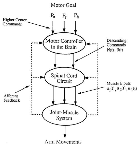
**Fig. 1.** The hierarchical structure of the model for movement control. The computation of motor commands is completed in two separate stages. The motor program located in the brain accepts inputs from higher centers of the brain and computes descending commands, which are then translated into muscle control inputs by a spinal cord circuit. Muscle inputs drive the arm to initiate a movement
